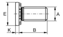
Head diameter E = 10.0 Head height K +/-0.02 = 1.50 Hole diameter +0.1 = 6 Length B +/-0.4 = 30 Male thread A = M6 Min distance to edge = 11.5 Tightening (N m) = 10.0
